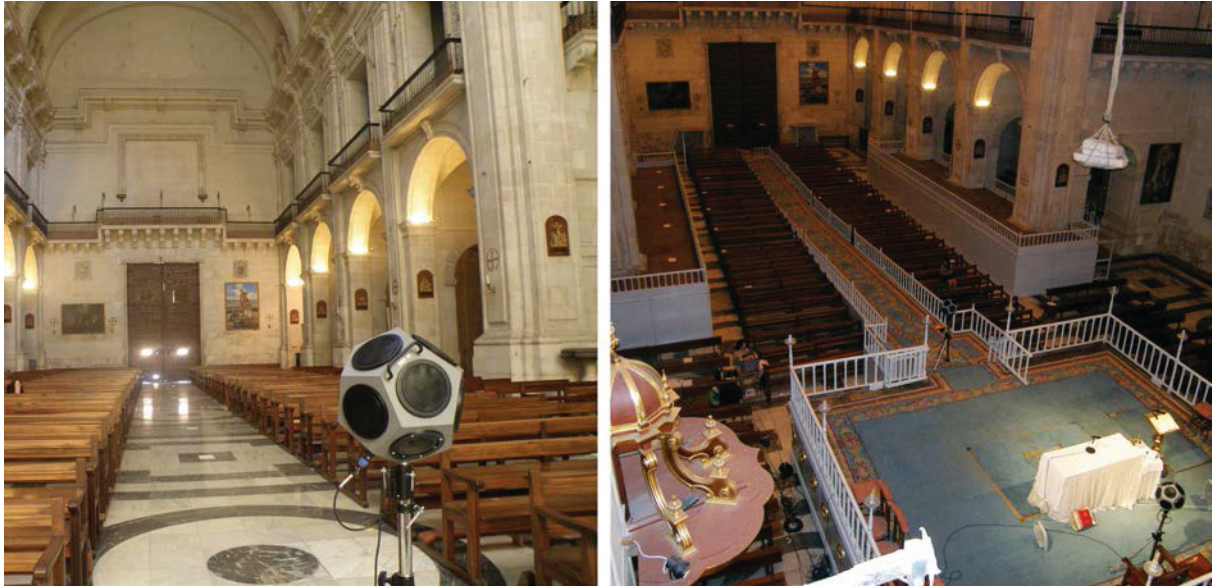
Figure 2. Measurement of acoustic parameters in the Basilica for both configurations.
